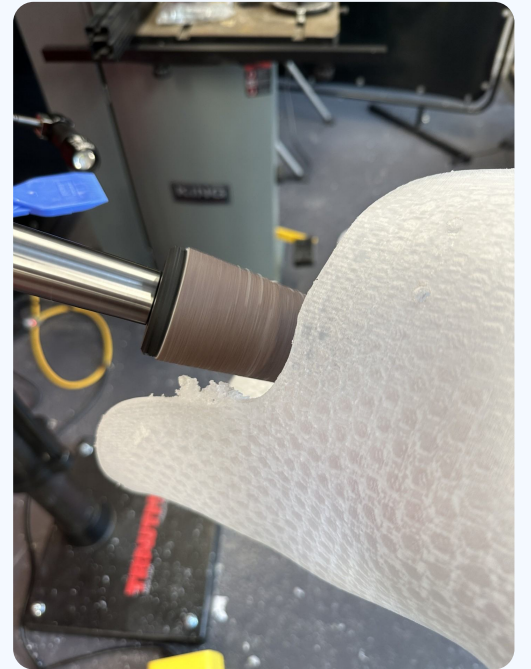
Material melting using a router
