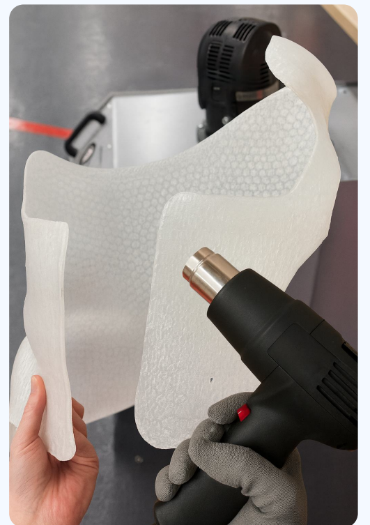
Hold heat gun 7–10 cm from surface
