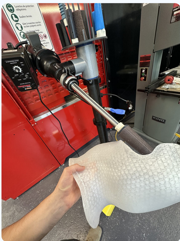
Second pass with P120 cone
